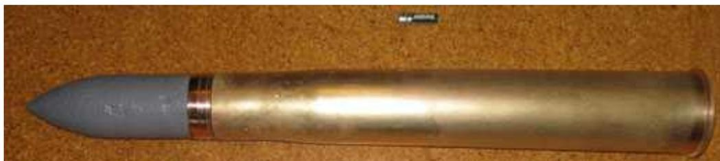
14 pdr projectile (in undercoat grey) and shell casing (800 mm) with AA battery for scale.<sup>11</sup>
